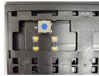
Amber LEDs (4) blinking when pairing
